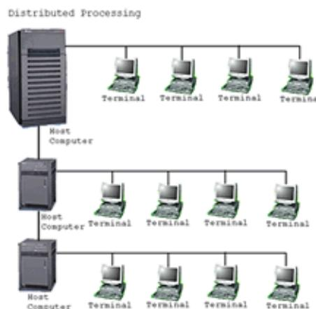
Gambar 2.2. Jaringan komputer model distributed processing.
